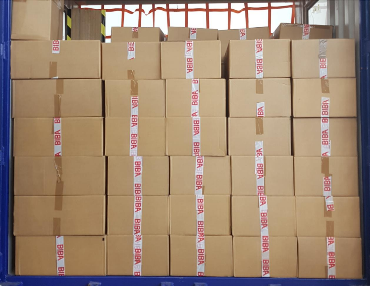
Figure 4: Pattern of a carton layer in a standard sea container as used in the tests.
