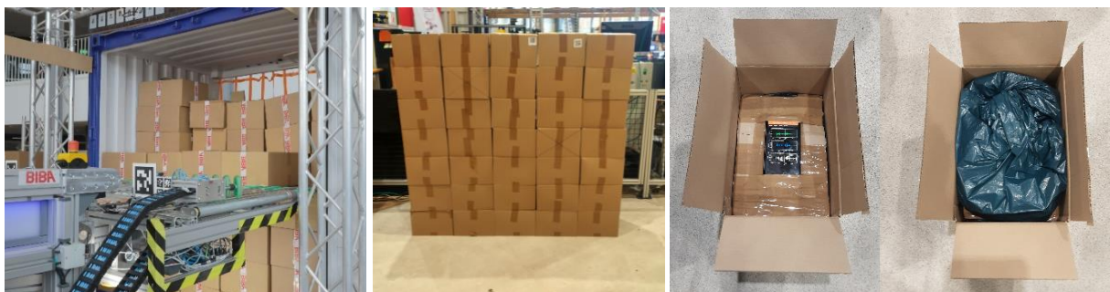
Figure 7: Experimental setup – developed container unloading system in front of container (left), bulk tests (middle) using parcels equipped with an accelerometer and additional weight (right)
