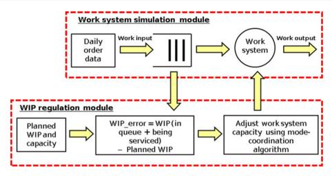
Fig. 3 Discrete event simulation of work system with autonomous WIP regulation
