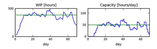
WIP regulation is not as effective as in the no-delay case, but capacity adjustment magnitudes are reduced. Again, the standard deviation of capacity and WIP are shown in Table 1.
