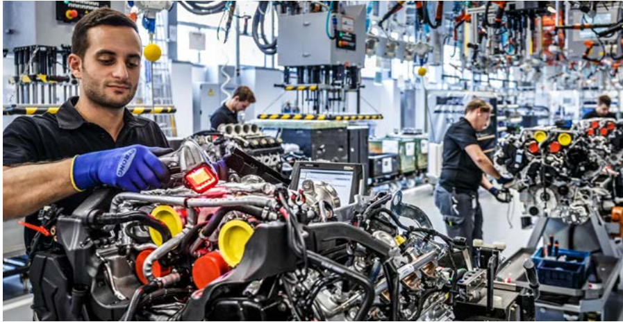
“One man, one engine” in the production of Mercedes-AMG
