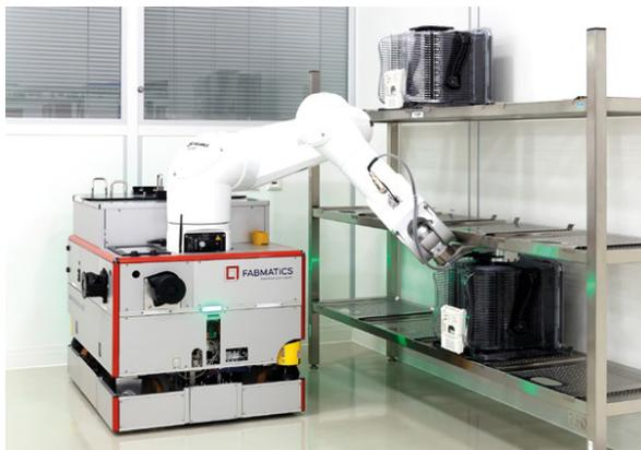
Figure 2: Multiple-load AGV equipped with a robot arm handling at a shelf in a semiconductor production facility (reference: [www.fabmatix.com](http://www.fabmatix.com))
