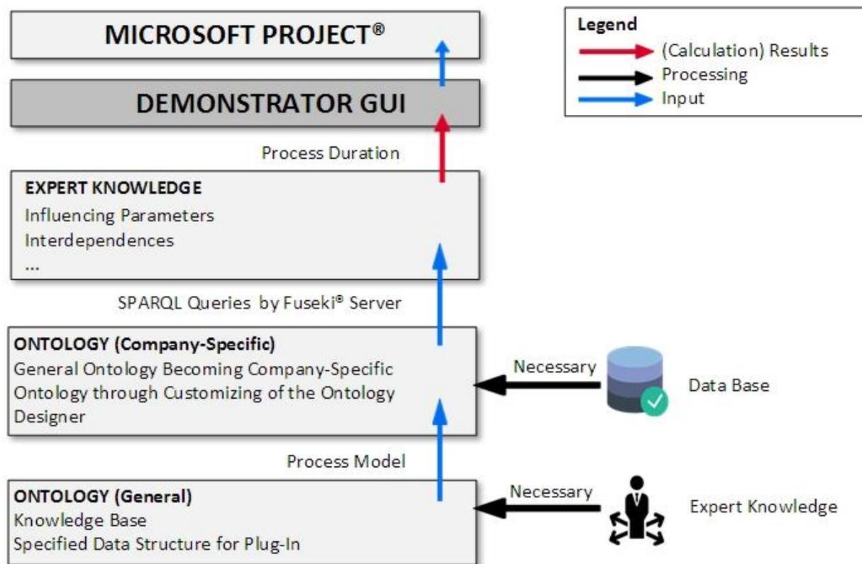
Figure 21: System architecture of the demonstrator
