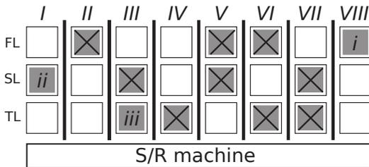
Figure 5: Triple-deep AS/RS after the second relocation.
