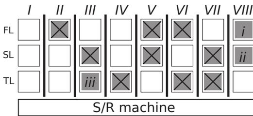
Figure 4: Triple-deep AS/RS after the first relocation.
