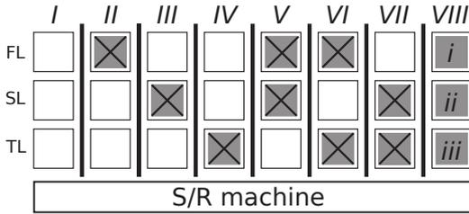
Figure 3: Triple-deep AS/RS. Storage good  $i$  shall be retrieved out of channel III.
