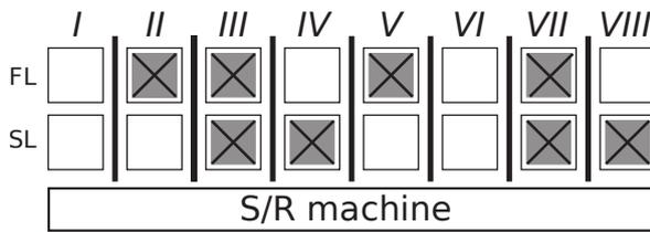
Figure 2: Example of a double-deep AS/RS.
