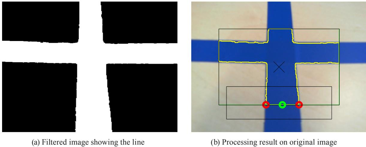
Figure 7: Line-following example using a blue line
