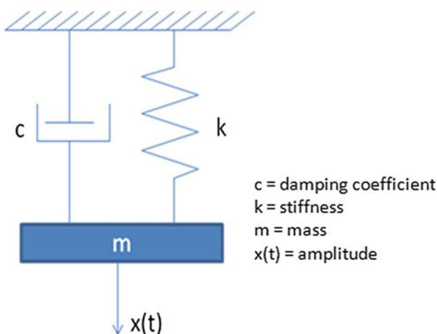
**Fig. 2** Fundamental elements of a vibratory system
