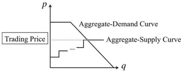
**Fig. 8** Determining the trading price under Mechanism 1
