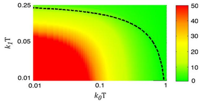
**Fig. 2** Normalized settling time  $T_s/T$  in response to turbulence versus  $k_0T$  and  $k_1T$
