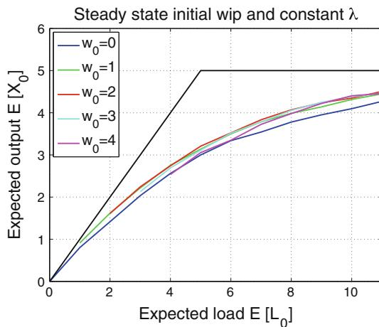
**Fig. 3** Expected ouflux for an  $M/M/1$  queue as in Fig. 1. Here, the ouflux represents an ensemble average over a steady-state probability distribution for the initial wips with a mean as indicated
