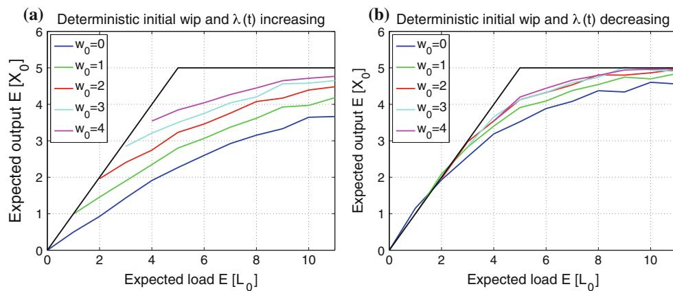
**Fig. 2** Clearing functions for an  $M/M/1$  queue with different initial wips and (a) increasing, (b) decreasing influx protocols
