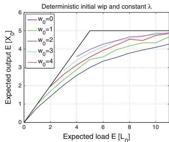
**Fig. 1** Expected total ouflux for an  $M/M/1$  queue for a time interval of five mean cycle times as a function of the expected total load
