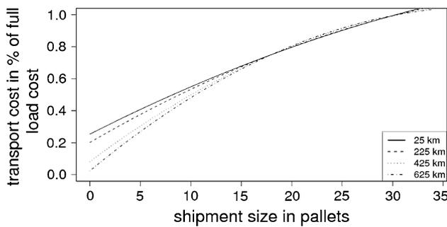
**Fig. 1** Proportion of full-truck load cost in function of shipment size
