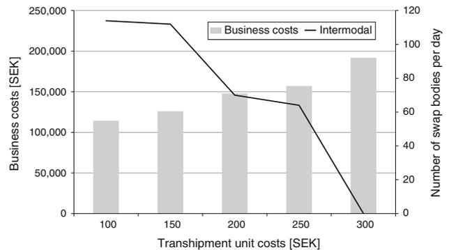
Fig. 7 Total business costs of the entire transport system for different TUC. The bars show the business costs (left axis). The line shows the number of swap bodies transported by the intermodal alternative (right axis)
