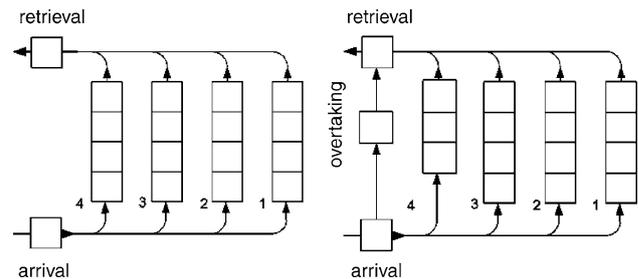
**Fig. 6** Example of mixed-bank buffers with and without overtaking lane [14]
