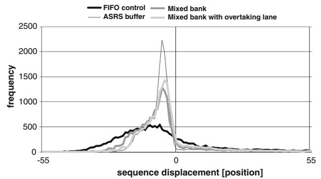
**Fig. 7** SD-distribution plot of the re-sequencing results of different buffer configurations [14]
