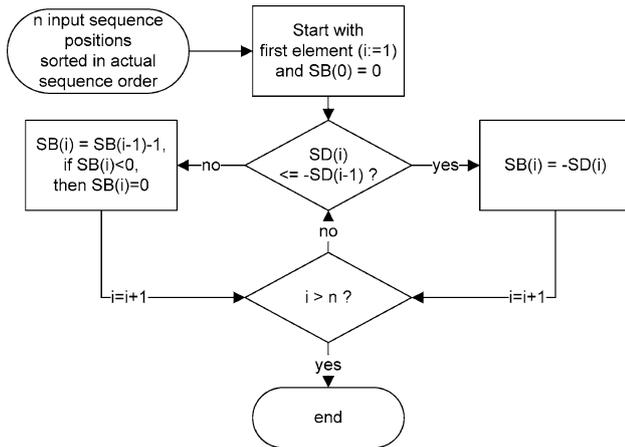
Fig. 5 Algorithm for calculation of the sequence backlog [14]
