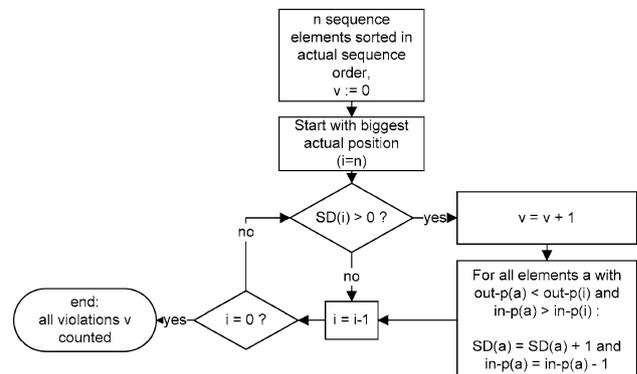
Fig. 4 Algorithm for calculation of sequence violations by means of the sequence displacement [14]
