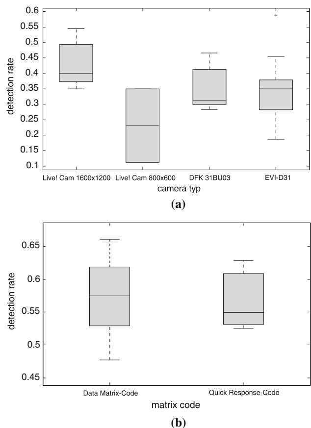
**Fig. 8** A quantitative comparison of the detection rates relating to (a) the camera type and (b) the marker types
