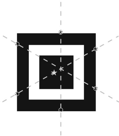
**Fig. 6** Finder pattern of a Quick Response marker (cf. Fig. 5). The midpoint of the finder pattern determined by a contour detection is marked by the intersection of the scanlines. The mean square error of the three scanlines is represented by the asterisk
