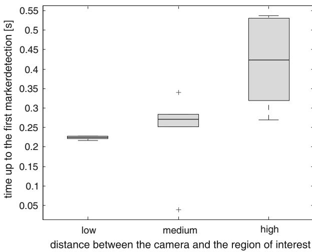
**Fig. 7** Comparison of different distances between the camera and the region of interest. The distinction is drawn between low (up to 1 m), medium (ca. 2 m), and high (from 3 m)
