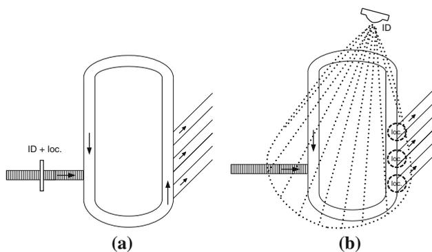
**Fig. 1** Identification and localization at a (a) central identification point, (b) global identification via RFID for the entire system, respectively for a bigger section and localization by vision at local intersection points
