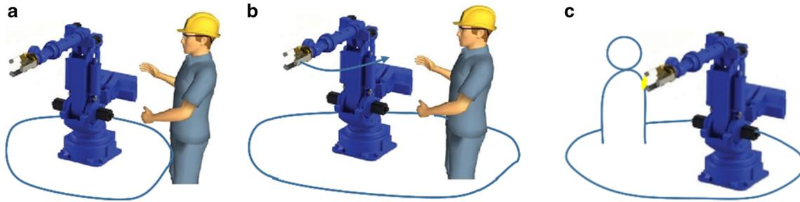
**Fig. 2** Collaboration classifications: **a** robot on safe hold against human violation, **b** speed reduction if the worker is in the robot work zone, **c** robot touching the human with a pre-defined calibrated force
