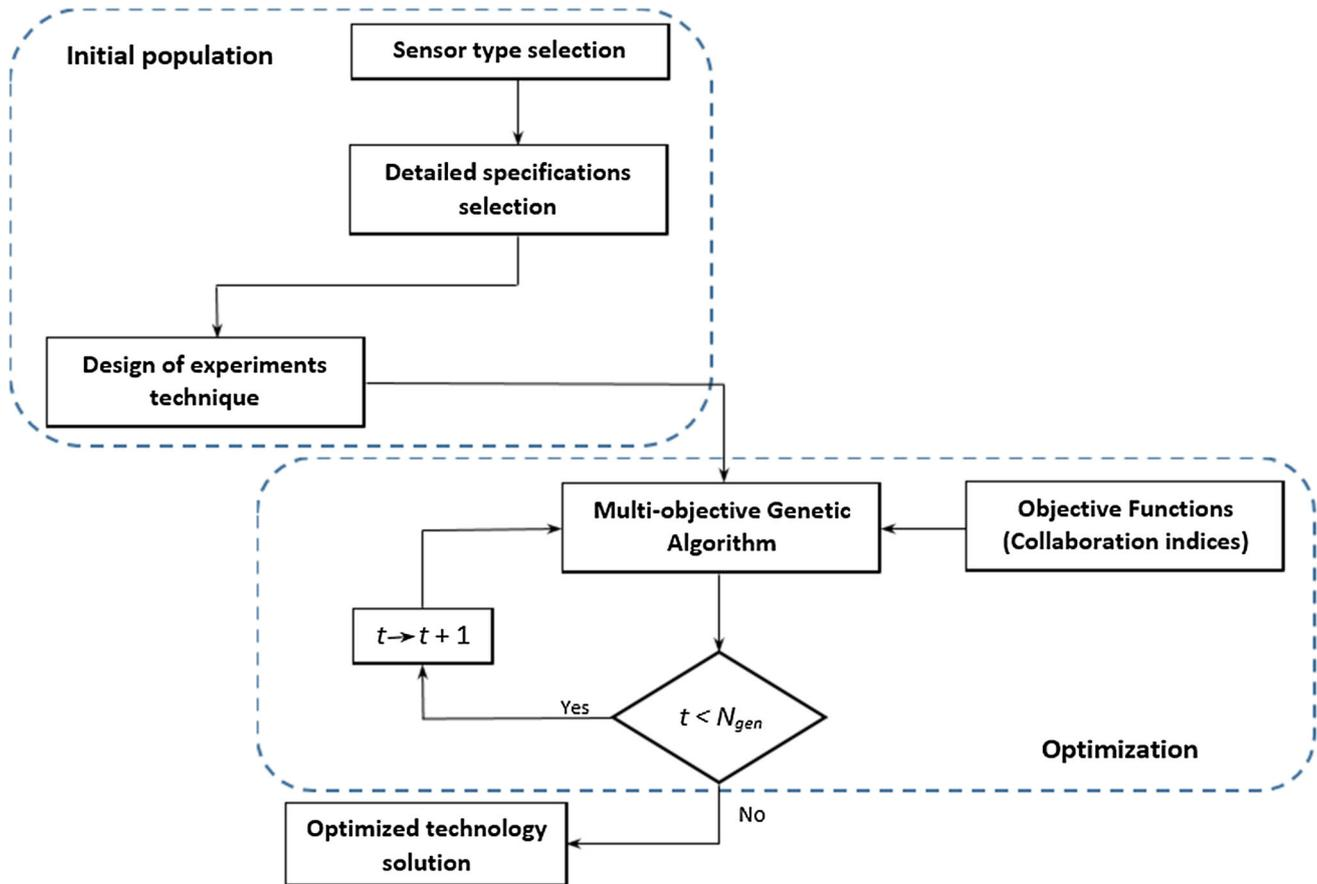
**Fig. 6** Optimization data flow in CRCPS design methodology
