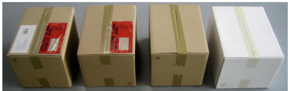
(a) Test objects with different material properties and the dimensions 380 \times 280 \times 280 mm (brown parcels) and 400 \times 300 \times 260 mm (white parcel).
